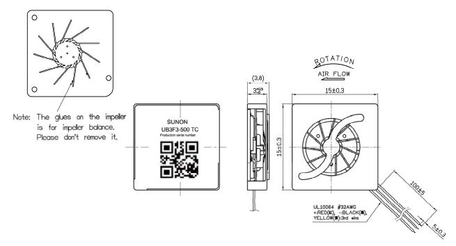
Marking (By laser): SUNON UB3F3-500 TC:Model name Production serial number:0Y17xxxxxx 0:Printing Plant Code Y:Manufacture Plant 17:Year,2017=17 xxxxxx: Producing Lot No. QR code:Content according to SUNON QR code specification TC:CUSTOMER NUMBER
